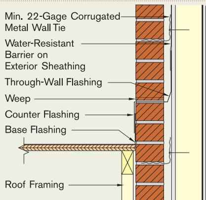
**Through-Wall Flashing at Roof Interface**
