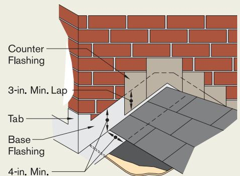
**Flashing at Roof /Chimney Intersection**
